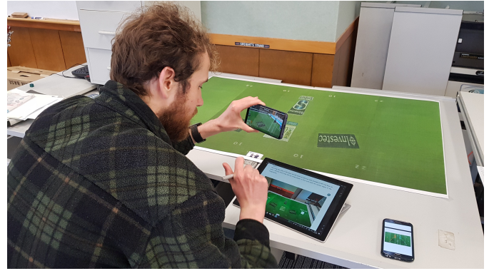
Fig. 5. A user study participant using the Lab AR prototype. Also seen is the smartphone (hand-held) to view the situated infographics and the other smartphone (on table) displaying traditional infographics.
